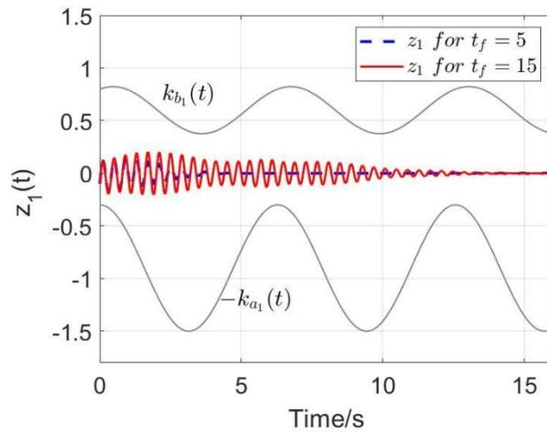
Fig.2. Tracking error trajectory
